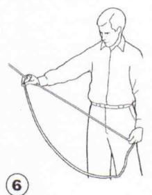
On opposite end of the guy rope slide wood peg up rope to create a loop.
